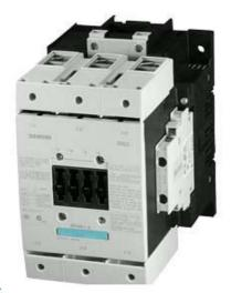
CONTACTOR, 55KW/400V/AC-3 AC(40...60HZ)/DC OPERATION UC 220...240V AUXIL. CONTACTS 2NO+2NC 3-POLE, SIZE S6 WITH BOX TERMINALS CONVENTIONAL OPERATING MECHAN. SCREW TERMINAL
