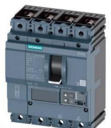
CIRCUIT BREAKER 3VA2 IEC FRAME 100 BREAKING CAPACITY CLASS L ICU=150KA @ 415 V 4POLE, LINE PROTECTION ETU860, LSIG, IN=40A OVERLOAD PROTECTION IR=16A ...40A SHORT CIRCUIT PROTECTION ISD=0,6..10X IN, II=1,5..12X IN NEUTRAL PROTECTION ADJUSTABLE (OFF, UPTO 160%) GROUNDFAULT, SWITCHABLE IG=0,2... 1 X IN, TG=0,050,8MS BUSBAR CONNECTION
