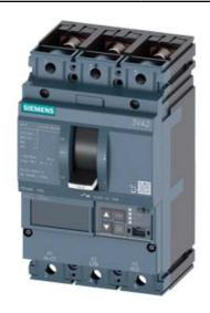
CIRCUIT BREAKER 3VA2 IEC FRAME 160 BREAKING CAPACITY CLASS M ICU=55KA @ 415 V 3POLE, LINE PROTECTION ETU860, LSIG, IN=100A OVERLOAD PROTECTION IR=40A ...100A SHORT CIRCUIT PROTECTION ISD=0,6..10X IN, II=1,5..12X IN NEUTRAL PROTECTION OPTIONAL WITH EXT. CT,UPTO 160% GROUNDFAULT, SWITCHABLE IG=0,2... 1 X IN, TG=0,050,8MS BUSBAR CONNECTION
