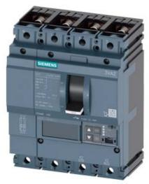
CIRCUIT BREAKER 3VA2 IEC FRAME 160 BREAKING CAPACITY CLASS M ICU=55KA @ 415 V 4POLE, LINE PROTECTION ETU850, LSI, IN=25A OVERLOAD PROTECTION IR=10A ...25A SHORT CIRCUIT PROTECTION ISD=0,6..10X IN, II=1,5..12X IN NEUTRAL PROTECTION ADJUSTABLE (OFF, UPTO 160%) BUSBAR CONNECTION
