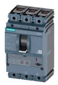
CIRCUIT BREAKER 3VA2 IEC FRAME 160 BREAKING CAPACITY CLASS L ICU=150KA @ 415 V 3POLE, LINE PROTECTION ETU350, LSI, IN=25A OVERLOAD PROTECTION IR=10A ...25A SHORT CIRCUIT PROTECTION ISD=1,5... 10 X IR, II=12 X IN CABLE CONNECTION
