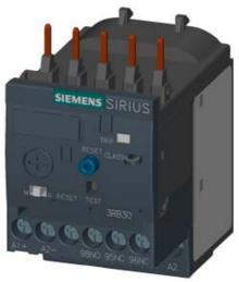
OVERLOAD RELAY 4...16 A FOR MOTOR PROTECTION SIZE S00, CLASS 20 CONTACTOR ASS. MAIN CIRCUIT: SCREW CONN. AUX.CIRCUIT: SCREW CONN. MANUAL-AUTOM.-RESET
