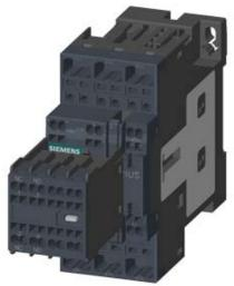
CONTACTOR, AC-3, 18.5KW/400V, 2NO+2NC, DC 24V, 3-POLE, SZ S0 SPRING-LOADED TERMINAL REMOVABLE AUX. SWITCH
