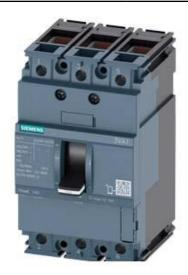
CIRCUIT BREAKER 3VA1 IEC FRAME 160 BREAKING CAPACITY CLASS H ICU=70KA @ 415 V 3-POLE, LINE PROTECTION TM210, FTFM, IN=100A OVERLOAD PROTECTION IR=100A FIXED SHORT CIRCUIT PROTECTION II=10 X IN CABLE CONNECTION
