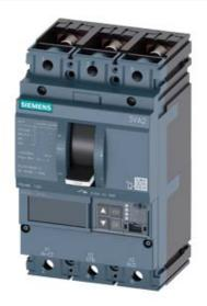
CIRCUIT BREAKER 3VA2 IEC FRAME 100 BREAKING CAPACITY CLASS H ICU=85KA @ 415 V 3POLE, LINE PROTECTION ETU550, LSI, IN=100A OVERLOAD PROTECTION IR=40A ...100A SHORT CIRCUIT PROTECTION ISD=0,6..10X IN, II=1,5..12X IN NEUTRAL PROTECTION OPTIONAL WITH EXT. CT,UPTO 160% BUSBAR CONNECTION
