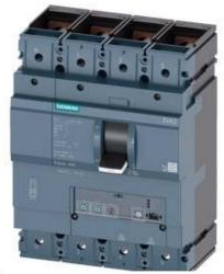
CIRCUIT BREAKER 3VA2 IEC FRAME 400 BREAKING CAPACITY CLASS C ICU=110KA @ 415 V 4-POLE, LINE PROTECTION ETU320, LI, IN=400A OVERLOAD PROTECTION IR=160A ...400A SHORT CIRCUIT PROTECTION II=10 X IN NEUTRAL PROTECTION ADJUSTABLE(OFF,50%,100%) BUSBAR CONNECTION
