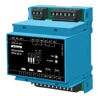
The current relay STW20V monitors the current in up to 3 lines with current transformers STWA 1 (AND circuit). If there is a current in all 3 monitored lines, the relay (2 change-over contacts) picks up. If there is no current in at least one of the lines, the relay releases.
