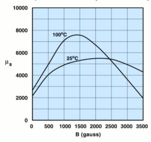
Measured on an 18/10/6mm toroid at 10kHz.
