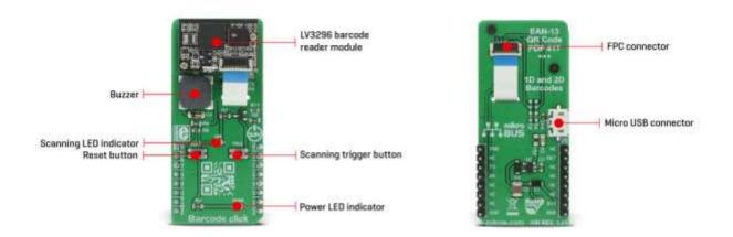
The LV3296 scanner module uses a flat cable to connect to the click board™, via the ZIF FPC connector on the back side of the PCB. This flat cable carries all the signals used in communication between the LV3296 module and the host MCU, such as the RX, TX, buzzer, USB, interrupt, reset, and scanning trigger lines.
