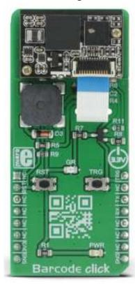
The barcode scanner module used for the Barcode click, is the <u>LV3296</u> made by Rakinda company, a compact barcode scanner module armed with the Rakinda patented UIMG® technology, designed to quickly scan the barcode and send the information either to the host MCU or the host PC. It also features an onboard speaker, used for signalization. These features make Barcode click an ideal solution for fast and accurate scanning of various types of barcodes.
