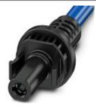
Photovoltaic connector, Range of articles: SUNCLIX, Photovoltaic connector, housing material: PPE, color: black, rated current: 20 A, Connection method: Crimp, Type of contact: Socket
