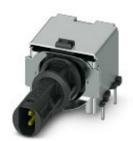
SPE PCB connector, type: IEC 63171-5, degree of protection: IP65/IP67, number of positions: 2, CAT B (ISO/ IEC 63171), connection method: THR solder connection, Single Pair Ethernet
