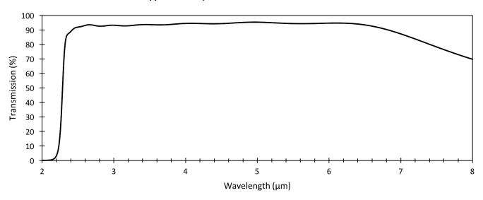
Typical 5.0 μm LP Filter Transmission
