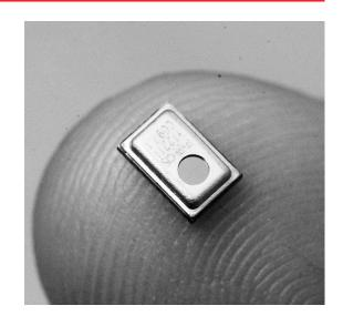
To make it easier for customers to use their own optical bandpass filters, Broadcom provides sensors with either a  $2.5-6~\mu m$  or  $6-14~\mu m$  broadband filter. Optical bandpass filters can be applied in front of these broadband filters.
