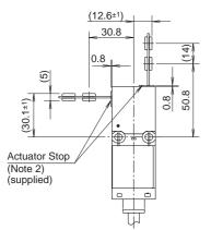
• Using the HS9Z-A62 Right-angle Actuator
