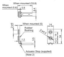
The orientation of actuator adjustment (horizontal/vertical) can be changed using the orienting insert (white plastic) installed on the
