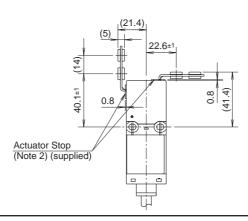
• Using the HS9Z-A65/A66 Angle Adjustable Actuator
