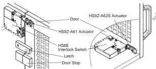
Note: When mounting an actuator, make sure that the actuator enters the slot in the correct direction, as shown on the right.
