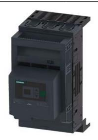
FUSE-SWITCH-DISCONNECTOR 3-POLE, NH00, 160A 40MM BUSBAR SYSTEM COVERS FOR RITTAL FLAT CONNECTOR FUSE MONITORING ELECTRONIC, EFM 20
