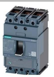
CIRCUIT BREAKER 3VA1 IEC FRAME 160 BREAKING CAPACITY CLASS H ICU=70KA @ 415 V 3-POLE, LINE PROTECTION TM220, ATFM, IN=32A OVERLOAD PROTECTION IR=22,4A ...32A SHORT CIRCUIT PROTECTION II=10 X IN BUSBAR CONNECTION
