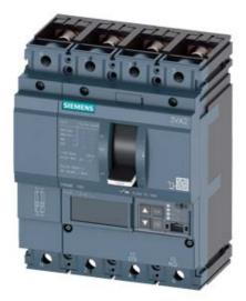
CIRCUIT BREAKER 3VA2 IEC FRAME 160 BREAKING CAPACITY CLASS C ICU=110KA @ 415 V 4POLE, LINE PROTECTION ETU550, LSI, IN=25A OVERLOAD PROTECTION IR=10A ...25A SHORT CIRCUIT PROTECTION ISD=0,6..10X IN, II=1,5..12X IN NEUTRAL PROTECTION ADJUSTABLE (OFF, UPTO 160%) BUSBAR CONNECTION
