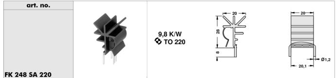
material: aluminium surface treatment: black anodised, solder pins tin plated
