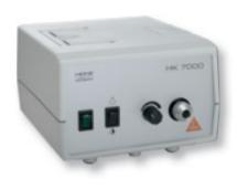
The F.O. Projector HK 7000 incorporates a special long-life halogen bulb rated at 150 Watts. If more light is needed for a particular examination, a boost switch can be operated, giving up to 40% more light. Suitable for all HEINE Systems with fiber optic illumination. Dimensions: Width 177 mm, Height 125 mm, Depth 217 mm. Weight 3,690 g.
