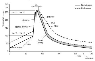
Soldering profile applied to a single soldering process.
