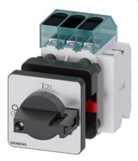
Switch disconnector 3LD3, main switch 3-polig, Iu 16A operational switch at AC-23 A at 400 V 7,5 kW front mounted Base mounting with center-hole 22,5 mm knob-operated mechanism black 48 x 48 mm with auxiliary 1NO+1NC
