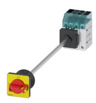
Switch disconnector 3LD3, main switch 3-polig + N, lu 25A operational switch at AC-23 A at 400 V 9,0 kW floor mounting Base mounting with door coupling center-hole 22,5 mm knob-operated mechanism red/yellow 48 x 48 mm
