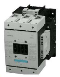
CONTACTOR, 55KW/400V/AC-3 AC(40...60HZ)/DC OPERATION UC 380-420V AUXILIARY CONTACTS 2NO+2NC 3-POLE, SIZE S6 WITH BOX TERMINALS CONVENTIONAL OPERATING MECHAN. CAGE CLAMP CONNECTION
