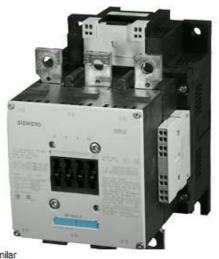
CONTACTOR, 160KW/400V/AC-3 AC(40...60HZ)/DC OPERATION UC 380-420V AUXILIARY CONTACTS 2NO+2NC 3-POLE, SIZE S10 BAR CONNECTIONS CONVENT. OPERATING MECHANISM CAGE CLAMP TERMINAL
