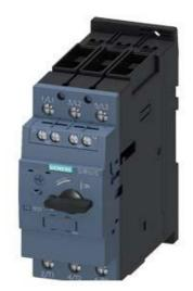
CIRCUIT BREAKER, SIZE S2, FOR MOTOR PROTECTION, CLASS 10, A-RELEASE 35...45A, N-RELEASE 650A, SCREW TERMINAL, STANDARD BREAKING CAPACITY W. TRANSV. AUX. SWITCH 1NO+1NC
