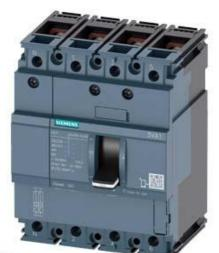
CIRCUIT BREAKER 3VA1 IEC FRAME 160 BREAKING CAPACITY CLASS N ICU=25KA @ 415 V 4-POLE, LINE PROTECTION TM210, FTFM, IN=100A OVERLOAD PROTECTION IR=100A FIXED SHORT CIRCUIT PROTECTION II=10 X IN NEUTRAL PROTECTION 50% BUSBAR CONNECTION
