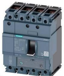
CIRCUIT BREAKER 3VA1 IEC FRAME 160 BREAKING CAPACITY CLASS H ICU=70KA @ 415 V 4-POLE, LINE PROTECTION TM240, ATAM, IN=25A OVERLOAD PROTECTION IR=17,5A ...25A SHORT CIRCUIT PROTECTION II=5...10 X IN NEUTRAL UNPROTECTED BUSBAR CONNECTION
