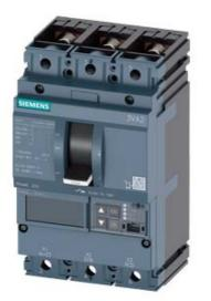
CIRCUIT BREAKER 3VA2 IEC FRAME 250 BREAKING CAPACITY CLASS H ICU=85KA @ 415 V 3POLE, LINE PROTECTION ETU550, LSI, IN=160A OVERLOAD PROTECTION IR=64A ...160A SHORT CIRCUIT PROTECTION ISD=0,6..10X IN, II=1,5..12X IN NEUTRAL PROTECTION OPTIONAL WITH EXT. CT,UPTO 160% BUSBAR CONNECTION
