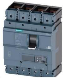
CIRCUIT BREAKER 3VA2 IEC FRAME 630 BREAKING CAPACITY CLASS H ICU=85KA @ 415 V 4-POLE, LINE PROTECTION ETU550, LSI, IN=400A OVERLOAD PROTECTION IR=160A ...400A SHORT CIRCUIT PROTECTION ISD=0,6..10X IN, II=1,5..15X IN NEUTRAL PROTECTION ADJUSTABLE (OFF, UPTO 160%) BUSBAR CONNECTION
