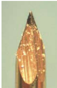
Standard Gold Coating, Contamination after 1/2 Mio contacts
