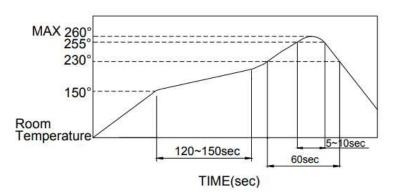
■ The temperatures defined above are the temperatures measured on the surface of the Printed Circuit Board. There are cases where the printed circuit board's temperature differs greatly from the temperature of the switch. Critical note: the switch's surface temperature must not exceed 260°C.
