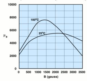
Measured on an 18/10/6mm toroid at 10kHz.
