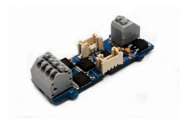
The LED Strip Driver with 4-pin Grove interface provides easy connectivity to your standard Arduino device or Seeed Stalker. It can help you control the luminance of a single-color LED strip, as well as the color and the luminance of an RGB LED strip through Arduino or Seeeduino.
