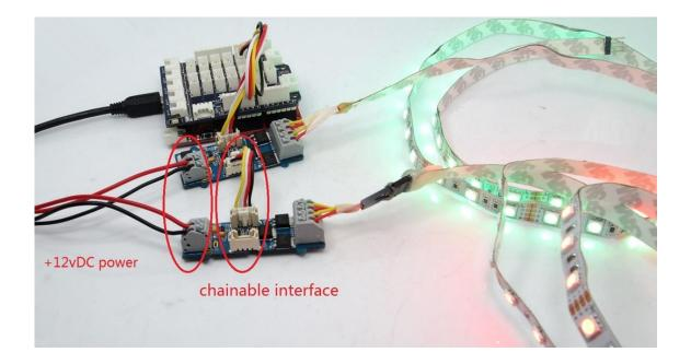
4.In cases that you want to utilize the cascade feature, prepare another driver and strip first. Then use a Grove cable to connect the Grove socket marked "out" on the first board and the Grove socket marked "IN" on the second board. Done. Two strips will shine in sync now.
