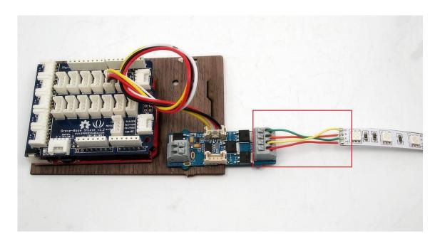
2.Connect the LED strip to the 4 pin terminal of Grove - LED Strip Driver. Make sure the wire marked "+12v" of the LED strip goes into
