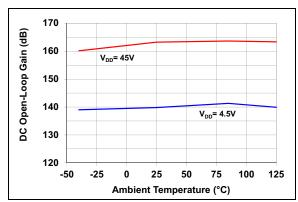
**FIGURE 2-12:** DC Open-Loop Gain vs. Ambient Temperature
