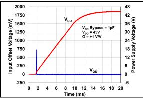
FIGURE 2-37: Input Offset Voltage vs. Time at Power-up
