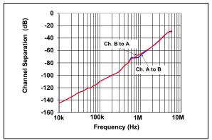
FIGURE 2-32: Channel-to-Channel Crosstalk (MCP6V52)
