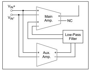
FIGURE 4-2: First Chopping Clock Phase; Equivalent Amplifier Diagram
