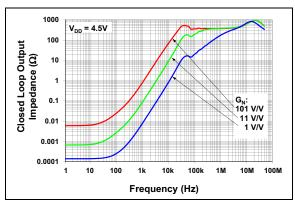
**FIGURE 2-28:** Closed-Loop Output Impedance vs. Frequency with  $V_{DD} = 4.5V$
