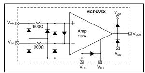
FIGURE 4-5: Simplified Analog Input ESD Structures
