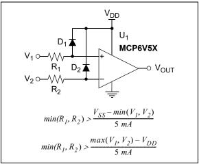
**FIGURE 4-7:** Protecting the Analog Inputs Against High Currents
