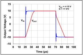
FIGURE 2-40: Noninverting Large Signal Step Response
