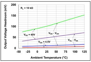
FIGURE 2-20: Output Voltage Headroom vs. Temperature RL = 10 kΩ
