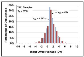
FIGURE 2-1: Input Offset Voltage
