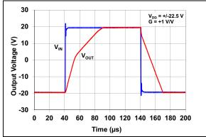
**FIGURE 2-41:** Noninverting 40 V<sub>PP</sub> Step Response
