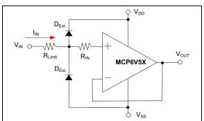
FIGURE 4-6: Protecting the Analog Inputs
