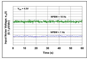
**FIGURE 2-34:** Input Noise vs. Time with 1 Hz and 10 Hz Filters and  $V_{DD} = 4.5V$
