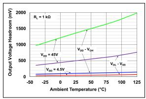
**FIGURE 2-19:** Output Voltage Headroom vs. Ambient Temperature
