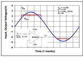
FIGURE 2-38: The MCP6V51/2/4 Shows No Input Phase Reversal with Overdrive
