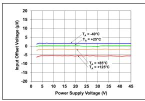
**FIGURE 2-3:** Input Offset Voltage vs. Power Supply Voltage
