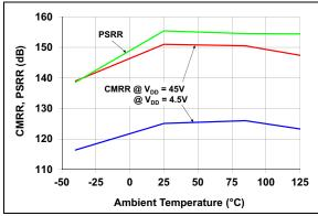
**FIGURE 2-11:** CMRR and PSRR vs. Ambient Temperature
