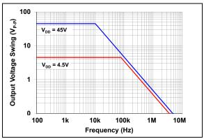
**FIGURE 2-30:** Maximum Output Voltage Swing vs. Frequency
