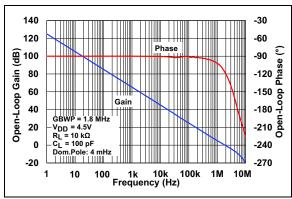
**FIGURE 2-24:** Open-Loop Gain vs. Frequency with  $V_{DD} = 4.5V$
