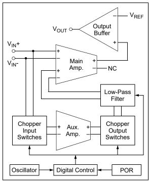
FIGURE 4-1: Simplified Zero-Drift Op Amp Functional Diagram
