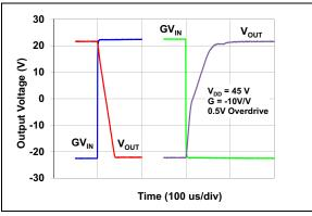
**FIGURE 2-46:** Output Overdrive Recovery vs. Time with G = -10 V/V
