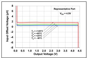
**FIGURE 2-4:** Input Offset Voltage vs. Output Voltage with  $V_{DD} = 4.5V$
