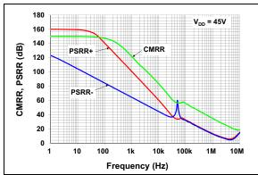
**FIGURE 2-23:** CMRR and PSRR vs. Frequency
