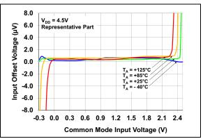
**FIGURE 2-6:** Input Offset Voltage vs. Common-Mode Voltage with  $V_{DD} = 4.5V$
