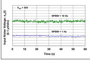
**FIGURE 2-35:** Input Noise vs. Time with 1 Hz and 10 Hz Filters and  $V_{DD} = 45V$
