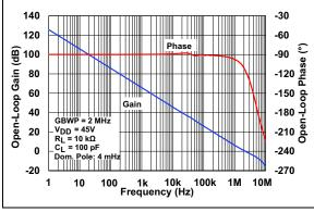
**FIGURE 2-25:** Open-Loop Gain vs. Frequency with  $V_{DD} = 45V$
