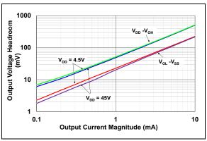
FIGURE 2-18: Output Voltage Headroom vs. Output Current
