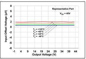
**FIGURE 2-5:** Input Offset Voltage vs. Output Voltage with  $V_{DD} = 45V$
