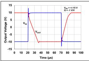
FIGURE 2-43: Inverting Large Signal Step Response
