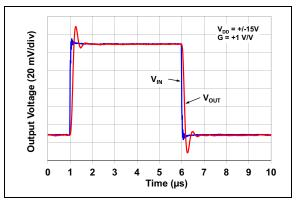
FIGURE 2-39: Noninverting Small Signal Step Response
