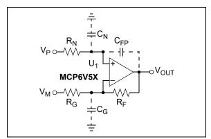
FIGURE 4-10: Amplifier with Parasitic Capacitance
