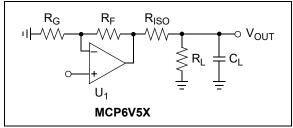
**FIGURE 4-9:** Output Resistor, R<sub>ISO</sub>, Stabilizes Capacitive Loads
