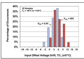
FIGURE 2-2: Input Offset Voltage Drift
