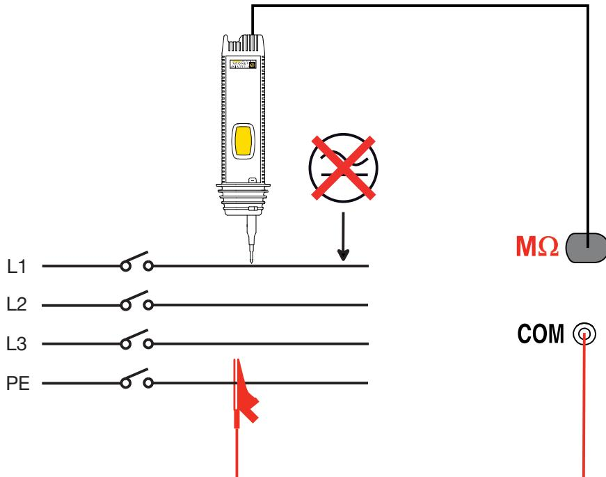
If it is dark, illuminate the measurement point by pressing the button underneath the probe.
