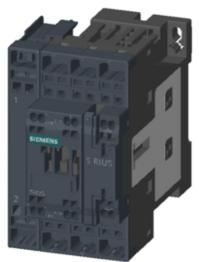
2NO+2NC CONTACTOR, AC3: 11KW DC 125V 4-POLE, 2NO+2NC, SZ: S0, SPRING-LOADED TERMINAL 1NO+1NC INTEGR.
