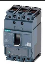
CIRCUIT BREAKER 3VA1 IEC FRAME 160 BREAKING CAPACITY CLASS M ICU=55KA @ 415 V 3-POLE, LINE PROTECTION TM220, ATFM, IN=100A OVERLOAD PROTECTION IR=70A ...100A SHORT CIRCUIT PROTECTION II=10 X IN CABLE CONNECTION
