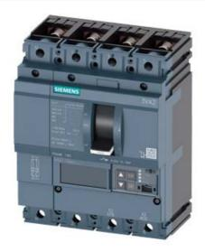
CIRCUIT BREAKER 3VA2 IEC FRAME 160 BREAKING CAPACITY CLASS C ICU=110KA @ 415 V 4POLE, LINE PROTECTION ETU860, LSIG, IN=160A OVERLOAD PROTECTION IR=64A ...160A SHORT CIRCUIT PROTECTION ISD=0,6..10X IN, II=1,5..10X IN NEUTRAL PROTECTION ADJUSTABLE (OFF, UPTO 100%) GROUNDFAULT, SWITCHABLE IG=0,2... 1 X IN, TG=0,050,8MS BUSBAR CONNECTION
