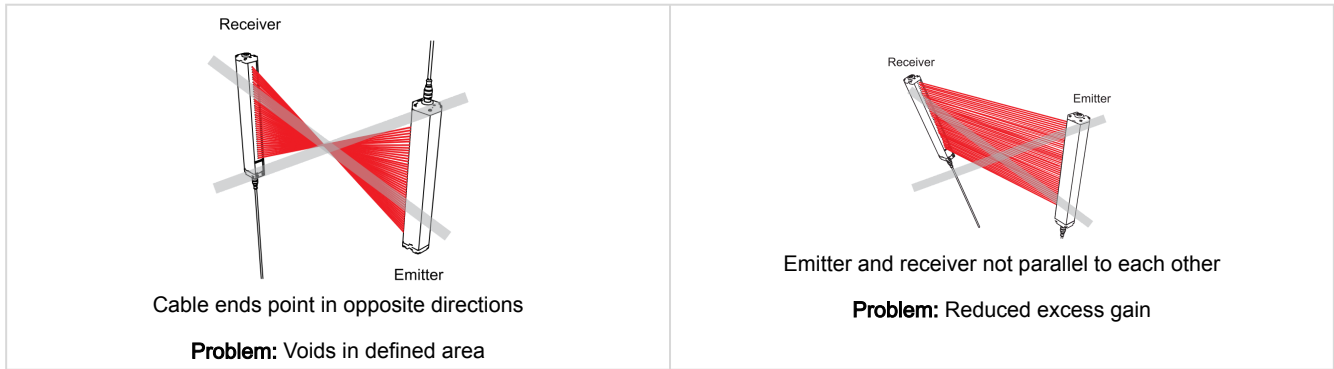
Figure 9. Examples of Incorrect Emitter/Receiver Orientation
