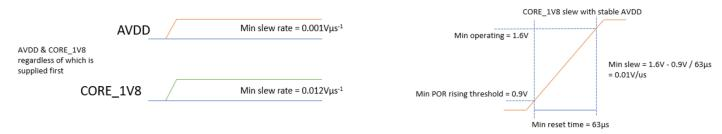
Note: The minimum reset time is the minimum time required for the device RAM to load and boot up after CORE\_1V8
