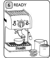
Discard the water from the pre-warmed cup or mug, dry and place back under the filter holder and your machine is ready to go.
