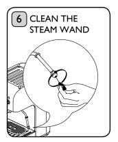
Use the steam pin to remove dried milk from inside the steam wand. Use the measuring spoon to place the nut back on the steam wand. Screw clockwise until tight.
