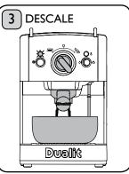
Place a large container on the drip tray. Operate as if making coffee. Continue until the tank is empty.
