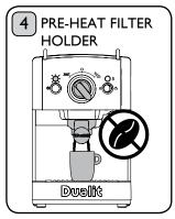
Dispense a mug full of water (min 240ml) through the machine. Ensure **NO** coffee is in the cup filter holder.
