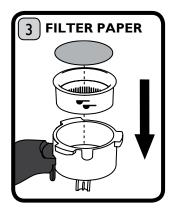
IMPORTANT NOTICE: Some very small coffee grounds can block the cup filters. To prolong the life of your machine use the enclosed filter papers with each serving.
