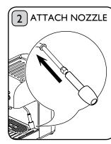
Put the froth nozzle on the end of the steam wand. Push up against the stopper shown above. Caution: Wand may be hot.
