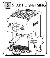
Turn the control knob to the steam/water position to start the water flowing. You will hear the pump; this is quite normal.
