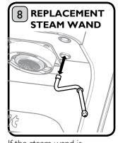
If the steam wand is completely blocked, it is possible to remove the wand assembly for cleaning. Visit our service section on www.dualit.com/support for replacement advise or to purchase spare parts.
