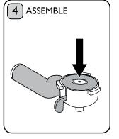
Lower the adapter to assemble and lock capsule in holder.
