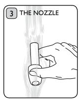
Pull the froth nozzle off the wand and wash under running water to remove any milk residue.
