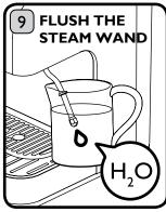
IMPORTANT NOTICE: Turn on your machine. Flush the steam wand by dispensing water or steam to remove any milk residue from inside the steam wand.
