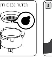
Select the ESE pod filter and snap into the filter holder.
