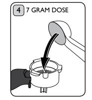
Using the measuring spoon, measure out one level spoon per serving into the cup filter. Use 2 level spoons if using the 2 cup filter.
