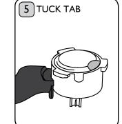
Make sure all the paper is tucked inside the filter before attaching the filter holder to the brewhead.
