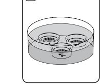
Place the filters in a container and soak in descaling solution.
