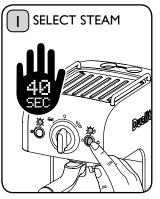
Set the steam/water selector to the steam setting. The temperature indicator will go out when the correct temperature has been reached.
