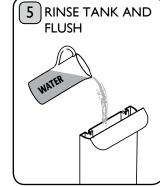
Rinse the water tank and fill with water. Operate as if making coffee and flush water through the machine. This will remove any traces of the descaling solution.
