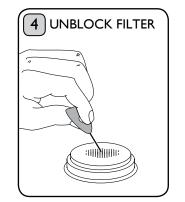
Filters often get blocked with prolonged use. To unblock, use the filter pin and push through the central hole on both sides of the filter to unblock.
