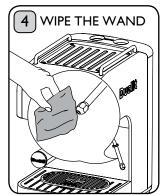
After each use, clean the wand with a damp cloth. There should be no milk residue visible.
