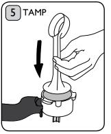
With the other end of the measuring spoon, 'tamp' the coffee grounds **LIGHTLY**. Tamping too hard, will stop water flowing through the ground coffee.
