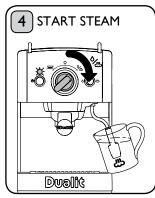
Turn the control knob to the steam position. You will hear the pump operating; this is quite normal. Steam will begin to flow.
