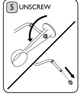
Locate the measuring spoon onto the steam wand nut. Unscrew anti-clockwise and remove.
