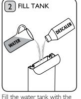
Fill the water tank with the descaling solution.
