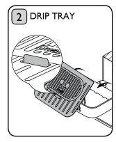
Empty the drip tray regularly. If the red tray full indicator is visable, empty immediately. Remove the non-slip mat and rinse after each use.
