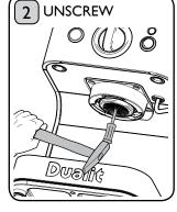
Using a screwdriver and hammer, **gently** tap the screw to dislodge any dried coffee. Then unscrew anti-clockwise.
