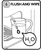
**IMPORTANT NOTICE:** After each use, flush the steam wand by dispensing water or steam to remove any milk residue from inside the steam wand. Wipe the steam wand.
