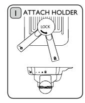
Align the holder with the open lock symbol, insert, then rotate 60° past the closed lock symbol.
