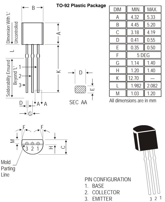
The TO-92 Package, Tape and Ammo Pack Drawings are correct as on the date of issue/revision of this Data Sheet.
