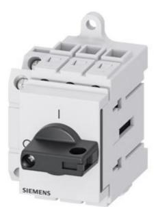
Switch disconnector 3LD3, main switch 3-polig, lu 32A operational switch at AC-23 A at 400 V 11,5 kW Distribution board mounting Base mounting with knob-operated mechanism black with auxiliary 1NO+1NC  $\,$
