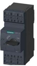
CIRCUIT-BREAKER SZ S0, FOR MOTOR PROTECTION, CLASS 10, A-REL. 1.4...2A, N-RELEASE 26A, SPRING-L. CONNECTION STANDARD SW. CAPACITY
