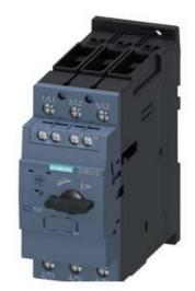
CIRCUIT BREAKER, SIZE S2, FOR MOTOR PROTECTION, CLASS 10, A-RELEASE 9.5...14A, N-RELEASE 208A, SCREW TERMINAL, STANDARD BREAKING CAPACITY W. TRANSV. AUX. SWITCH 1NO+1NC
