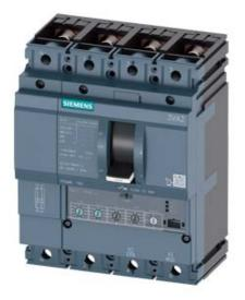
CIRCUIT BREAKER 3VA2 IEC FRAME 160 BREAKING CAPACITY CLASS M ICU=55KA @ 415 V 4POLE, LINE PROTECTION ETU350, LSI, IN=100A OVERLOAD PROTECTION IR=40A ...100A SHORT CIRCUIT PROTECTION ISD=1,5... 10 X IR, II=12 X IN NEUTRAL PROTECTION ADJUSTABLE(OFF,50%,100%) BUSBAR CONNECTION
