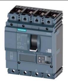
CIRCUIT BREAKER 3VA2 IEC FRAME 160 BREAKING CAPACITY CLASS C ICU=110KA @ 415 V 4POLE, LINE PROTECTION ETU550, LSI, IN=100A OVERLOAD PROTECTION IR=40A ...100A SHORT CIRCUIT PROTECTION ISD=0,6..10X IN, II=1,5..12X IN NEUTRAL PROTECTION ADJUSTABLE (OFF, UPTO 160%) BUSBAR CONNECTION
